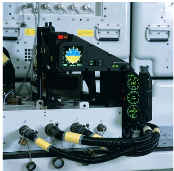
Fig. 6. GPATE TPS: UUT & Holding Fixture
