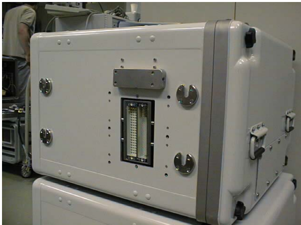
Fig. 5 . Example of Case Side with Floating Blind Mate and Alignment Pins (Female Type).
